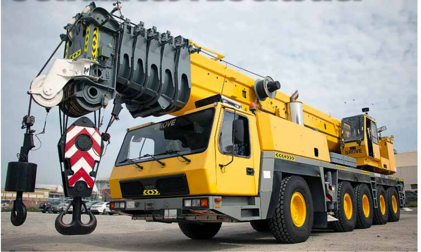
SembCorp's 2003 Grove GMK5200 All-Terrain-Kran.
